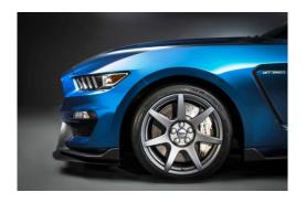
The two front wheels are insulated with a ceramic thermal barrier coating adapted from technology that is similar to what NASA used on the space shuttle. Each 19-inch carbon-fiber wheel weighs about 15 pounds less than an equivalently sized aluminum wheel,
