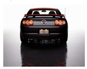
The combined suspension and tire package allows Boss to achieve a top speed of 155 mph and become the first non-SVT Mustang ever to achieve more than 1.0 g of lateral acceleration.
