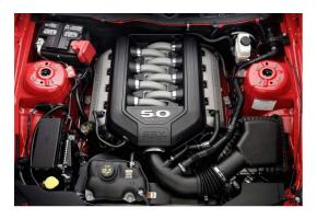
Performance and fuel economy The 412 horsepower and 390 ft.-lb. of torque delivered by the 2011 Mustang GT 5.0-liter V-8 represent significant increases versus the 2010 model year output levels.
