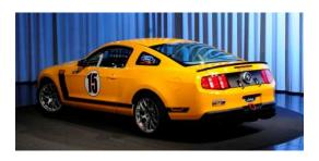
The Mustang BOSS 302R is a serialized off-road-only vehicle ready to race. Each base model will come with a 5.0-liter four-valve engine and a six-speed manual transmission with a roll cage, race seats, safety harness, data acquisition and race dampers/springs, and a Brembo brake and tire package, starting at an MSRP of \$79,000.
