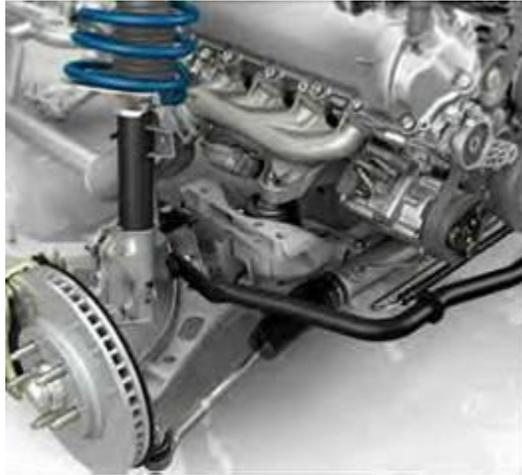
The MacPherson-strut front suspension's reverse "L" lower control arms are the product of a groundbreaking manufacturing technology used to produce steel control arms that actually weigh less than some comparable cast-aluminum designs. MacPherson struts originally developed in the 1940s by Earl S. MacPherson, a Ford engineer are widely renowned for their ability to deliver both comfort and control with reduced weight.
